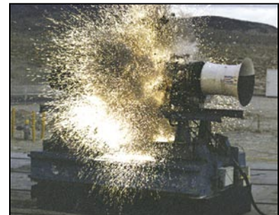
Figure 1. F404 ballistic test, uncontained failure
