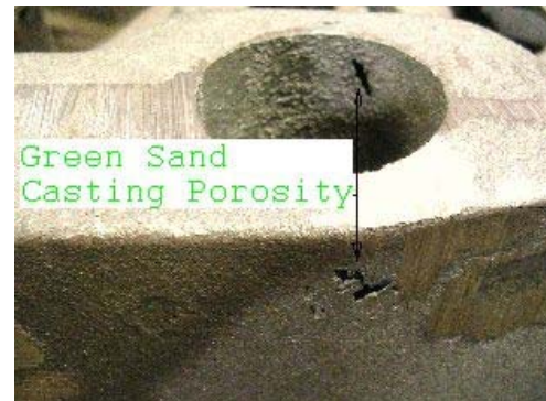
Figure 2-17: Close up of Through Wall Casting Defects
