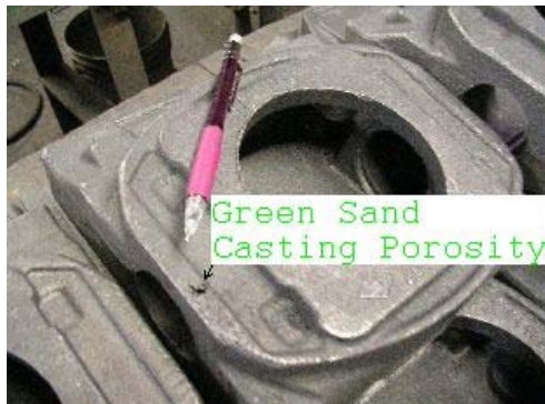
Figure 2-16: Through Wall Casting Defect
