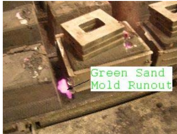
Figure 2-15: Mold Run Out
