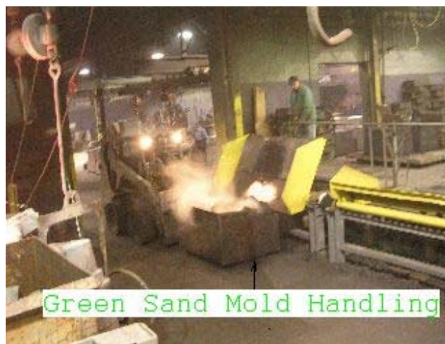
Figure 2-12: Handling of Hot Castings
