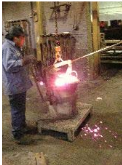
Figure 2-13: Temperature measurement of ladle
