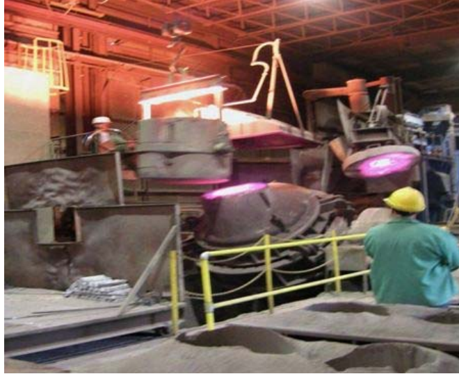
Figure 2-20 Crane Hook arrangement as ladle is poured into add vessel
