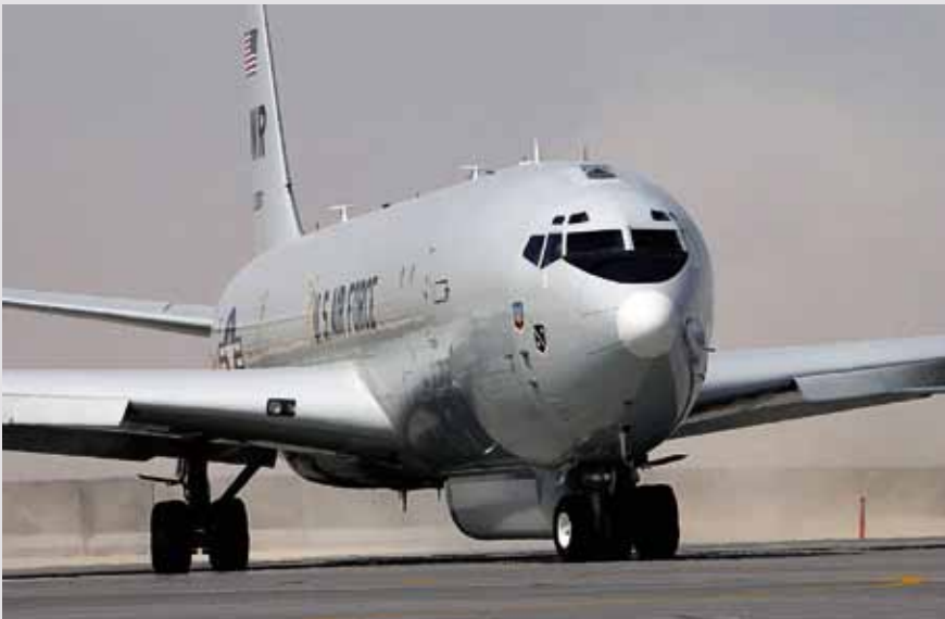
Figure 3. A U.S. Air Force E-8C Joint Surveillance Target Attack Radar System (Joint STARS) aircraft assigned to the 128th Expeditionary Air Command and Control Squadron. The Joint STARS is a battle management and command and control aircraft that tracks ground vehicles and some aircraft, collects imagery, and relays tactical pictures to ground and air theater commanders. U.S. Air Force photo by SSgt Aaron D. Allmon II.
