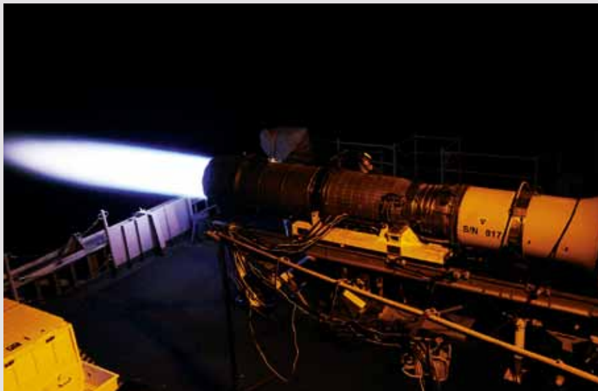
Figure 2. A U.S. sailor assigned to the aviation intermediate maintenance department's jet shop watches during a jet engine test cell on an F404-GE-400 jet engine for an F/A-18C Hornet aircraft on the fantail of aircraft carrier USS Nimitz (CVN 68), October 14, 2009, in the Indian Ocean. The F404 engine has twice won the Department of Defense Performance-Based Logistics Award. U.S. Navy photo by MC3 John Phillip Wagner Jr.
