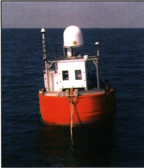
NRL's Satellite-Linked Vertical Line Array (SVLA) buoy during a recent ocean deployment. Data from an array of hydrophones are collected and stored within the buoy and simultaneously transmitted to both ships in the vicinity and distant shore stations using RF and satellite communications.
