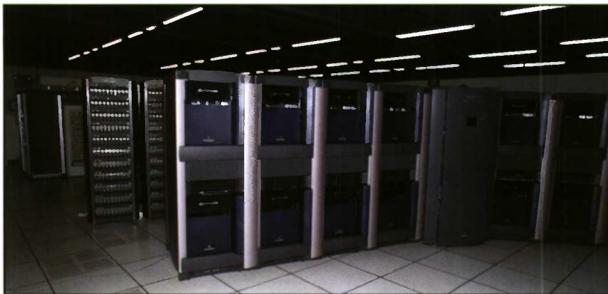
The 128-processor Silican Graphics Origin2000 system, currently with 128 Mbytes of RAM. The NRL Center for Computational Science, as a Distributed Center of the DoD High Performance Computing Modernization Program, provides such systems (at no cost) for anyone approved by the Program Office. The NRL CCS routinely upgrades high-end computing resources such as this.
