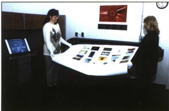
The Visual Imaging Services Section of the Technical Information Division has a color, wide-format Navajet Pro 600E printer and laminator that produces prints up to 60 inches wide, unlimited length, and at resolutions up to 600 dpi.
