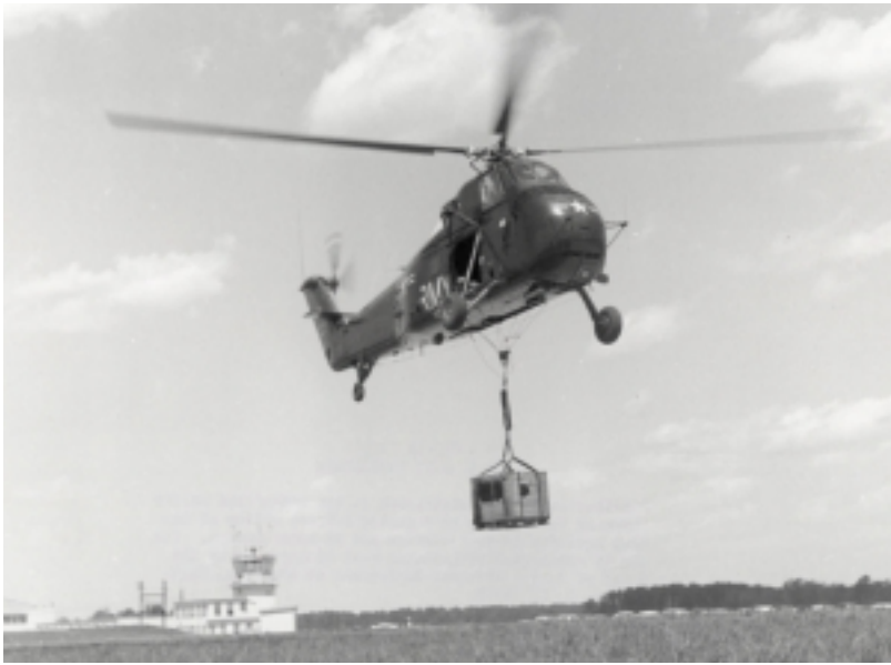
H-34 demonstrating pickup system at Fort Eustis, 1961.
