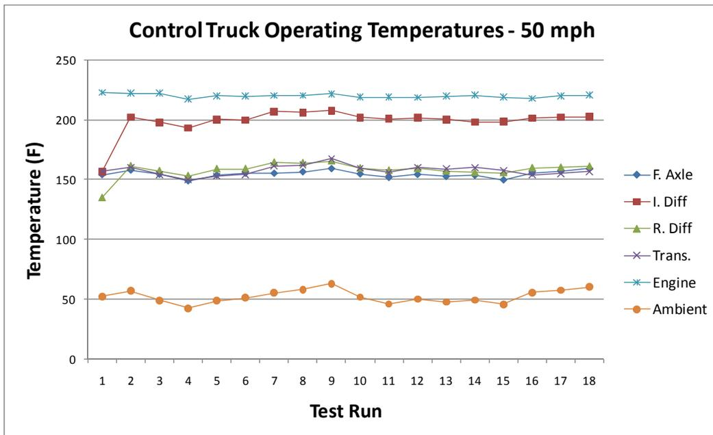
Figure B4. Control Truck Operating Temperatures – 50mph
