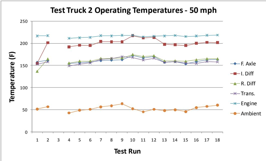
Figure B6. Test Truck 2 Operating Temperatures – 50mph
