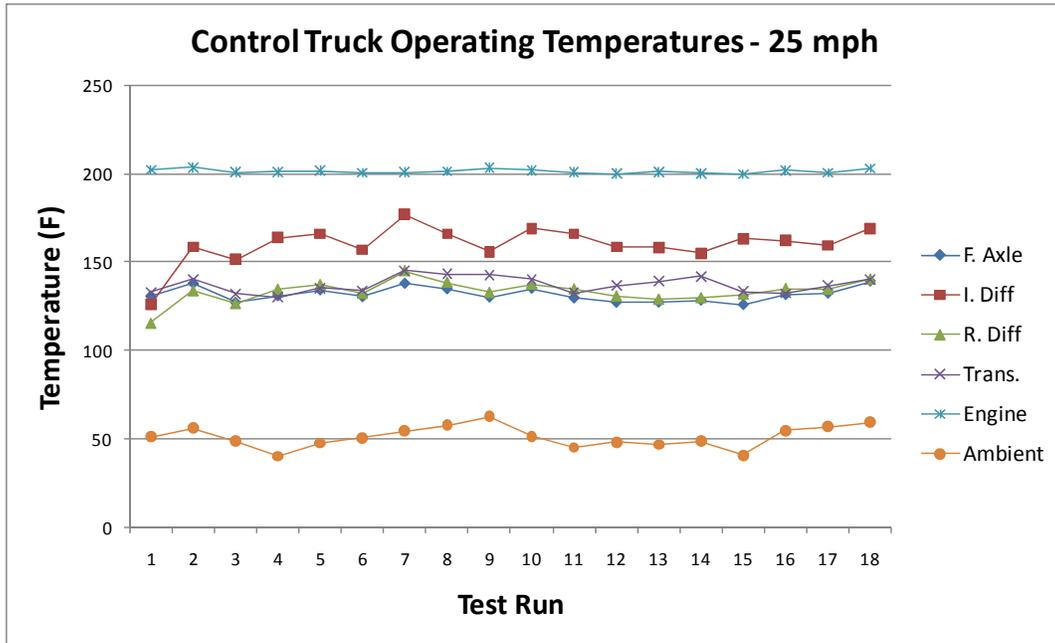
Figure B1. Control Truck Operating Temperatures – 25mph
