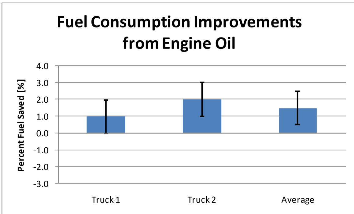
Figure 3: Fuel Consumption Improvement, MIL-PRF-2104G vs. MIL-PRF-46167D
