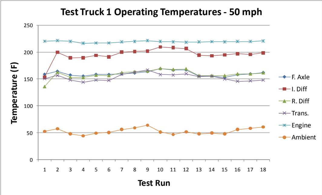
Figure B5. Test Truck 1 Operating Temperatures – 50mph
