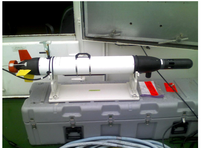
Fig. 2. The Iver2 AUV equipped with the YSI 6600 V2 sonde, Woods Hole Oceanographic Institute acoustic micromodem and a 16-element towed hydrophone array. The payload computer stack consists of a PIII-800 CPU and two 8 channel D/A boards. This model Iver2 navigates on the surface using GPS and underwater using a compass and speed table. This vehicle is designed for adaptive and collaborative autonomy experimentation applications including anti-submarine warfare and rapid environmental assessment.
