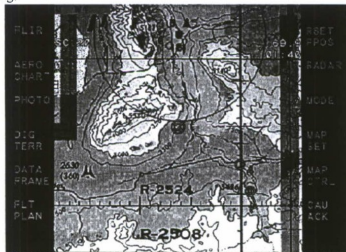
Figure 1. Example of a TAMMAC DMS baseline feature: Dynamic Display Overlay showing elevation color banding and threat rings.
