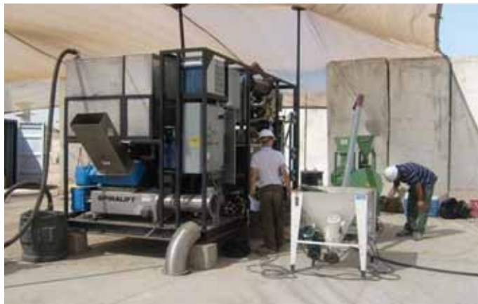
The Tactical Garbage to Energy Refinery being installed in Iraq.
