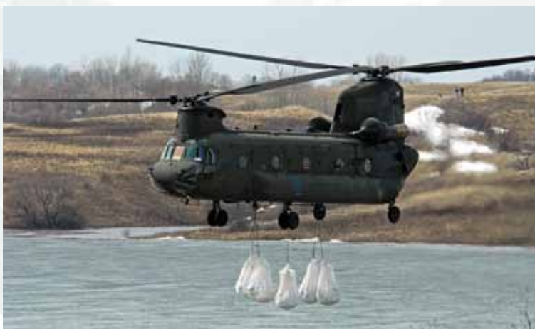
A North Dakota Air National Guard CH-47 Chinook helicopter drops several one-ton sandbags onto the spillway of the Clausen Springs Dam as part of a flood control effort.
