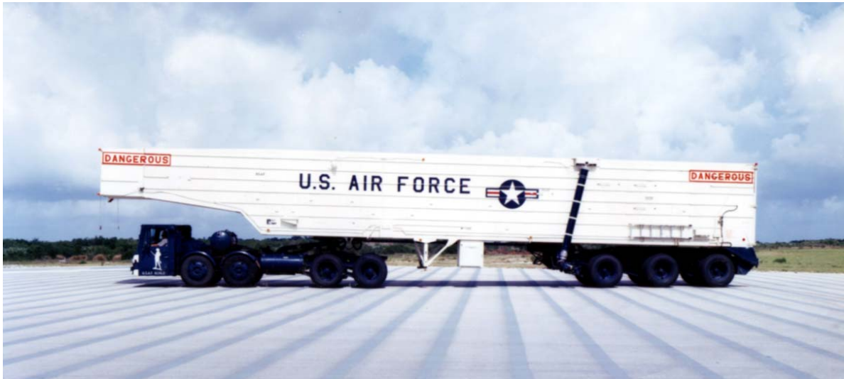
Figure 34. New transporter/erector for Minuteman, 1961 (NARA).
