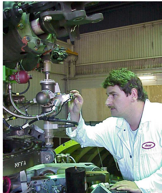
Fig. 3. IBC actuator installed in the rotor system.
