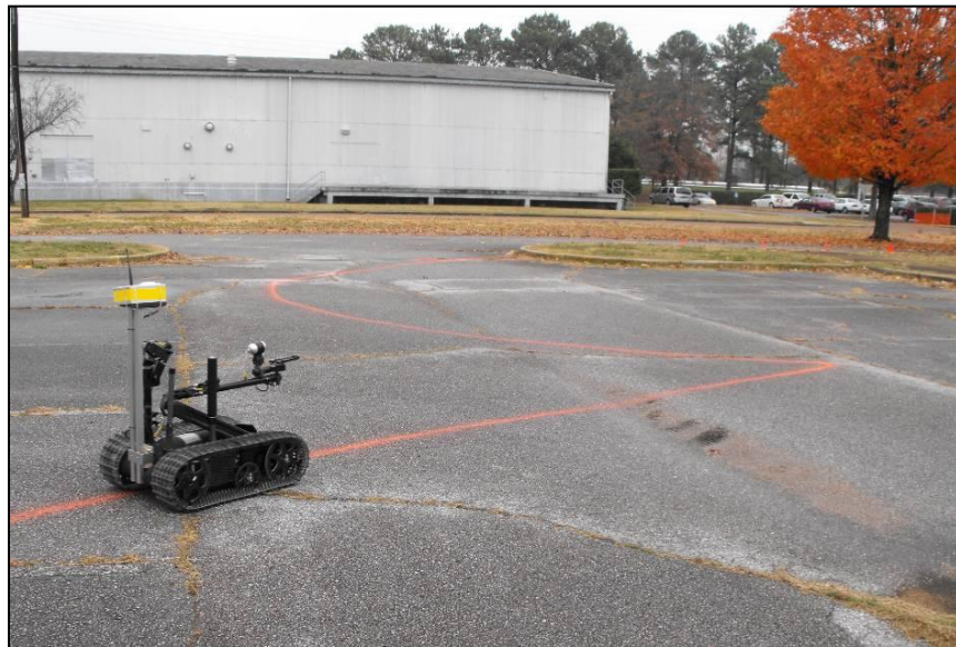
Figure 7. TALON on path following course.
