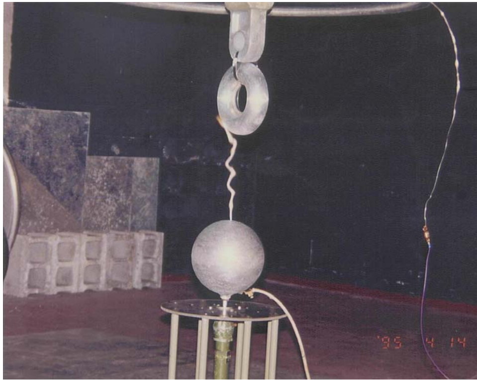
Figure 8-68. Arc current and voltage measurement test setup.
