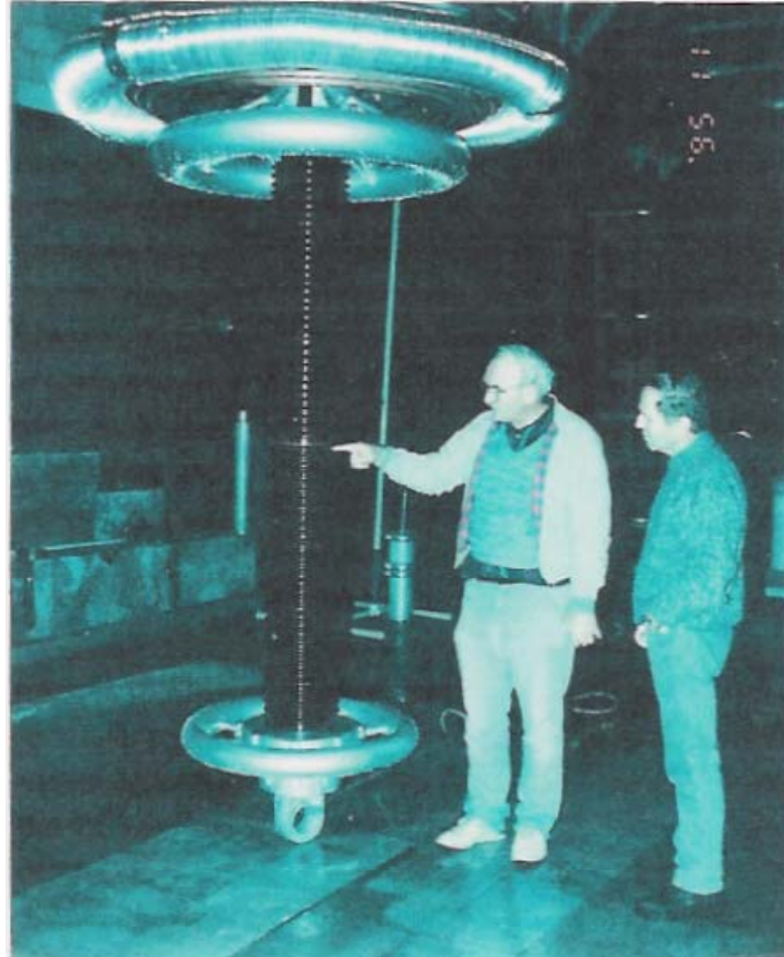
Figure 8-54. Mockup of large corona ring using corrugated pipe.
