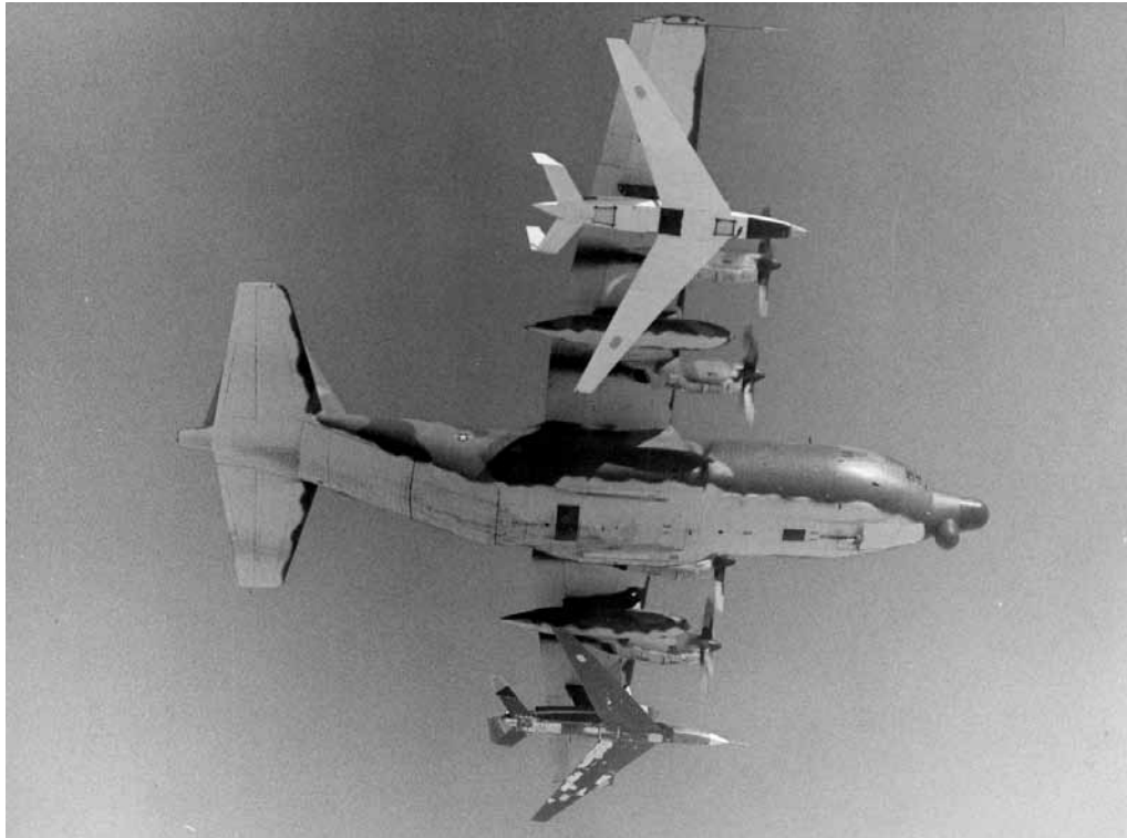
Teledyne Ryan Model 154 (USAF AGM-91) RPVs, known as Compass Arrow, carried aloft by a DC-130.
