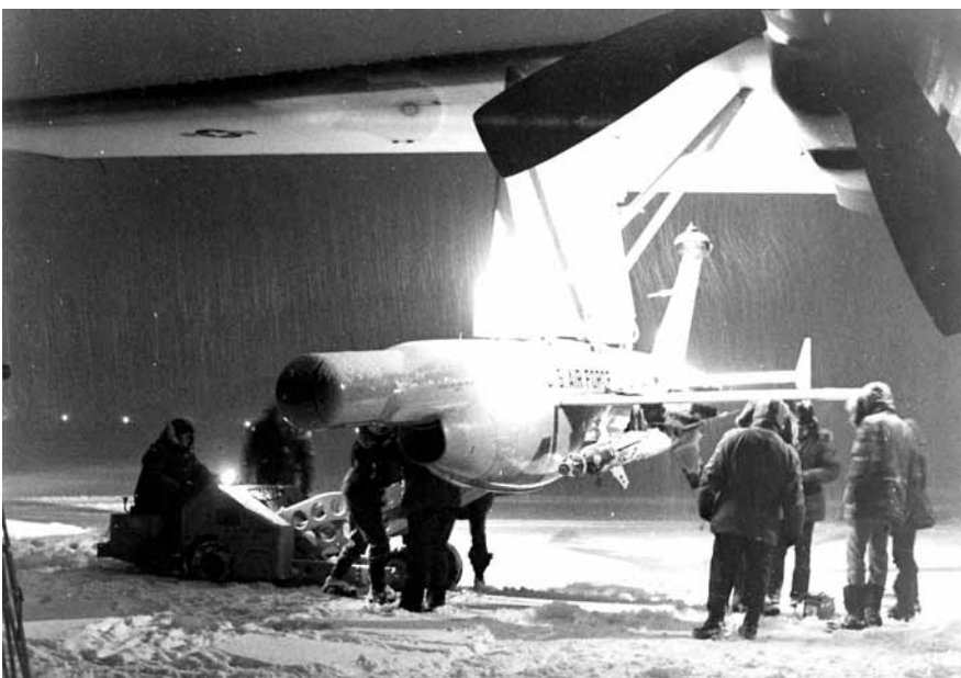
A BGM-34 RPV being loaded with two Mk-81 bombs at Hill AFB, Utah.
