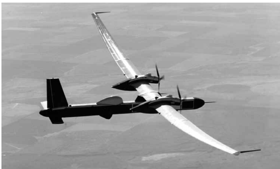
Boeing's high-altitude, long-endurance Condor UAV did not enter operational service but was important as a technology testbed.
