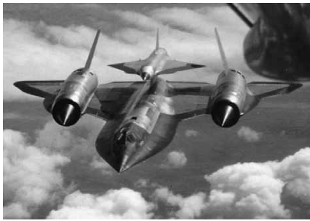
D-21 drone carried aloft by its mothership, a specially configured A-12, redesignated M-12 (also referred to as M-21).
