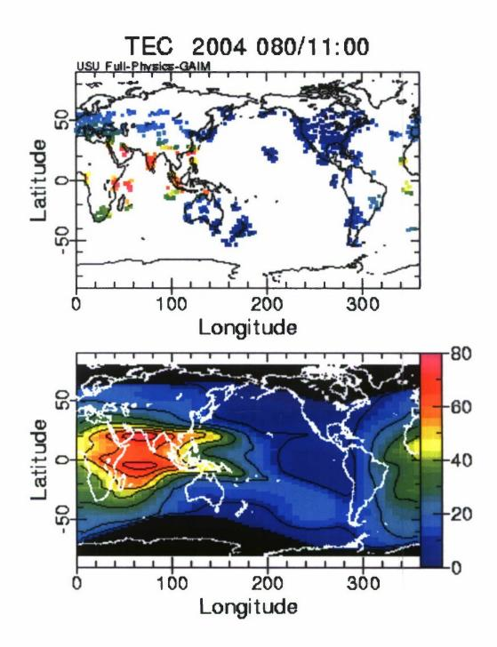
Figure 1. Distributions of vertical TEC obtained from GPS measurements (top) and the GAIM-FP model (bottom). The units are  $10^{16}$  el/m<sup>2</sup>.
