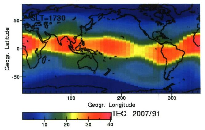
Figure 2. Example of a TEC map obtained from our Full Physics-Based Kalman filter model for April 1, 2007. The TEC values are shown for a fixed solar local time (SLT=1730). Clearly seen is the wave number-four structure in the low-latitude TEC distribution. From Scherliess et al., 2009.
