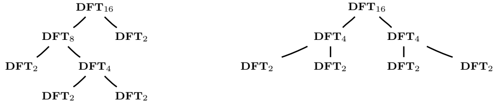
FIGURE 4.2: Two fully expanded ruletrees for \mathbf{DFT}_{16} .
