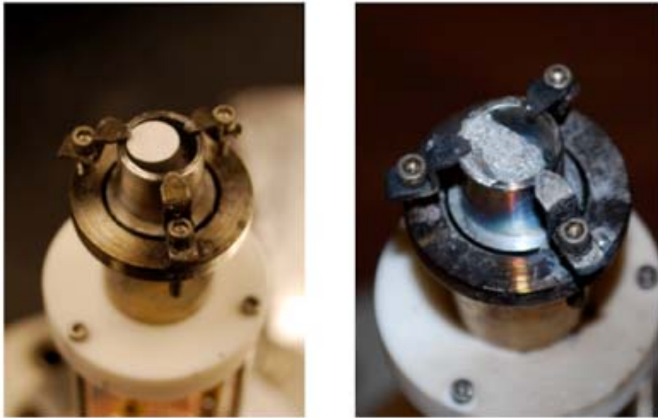
Figure 57. Aluminum sample before and after vapor deposition
