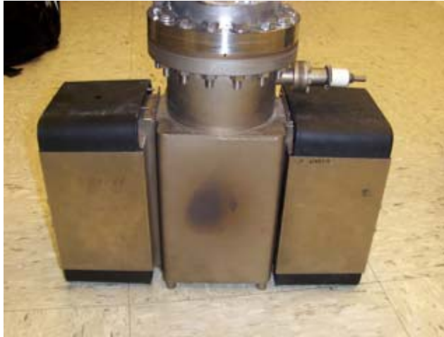
Figure 25. Ion Pump used for EIMAC cathode test stand
