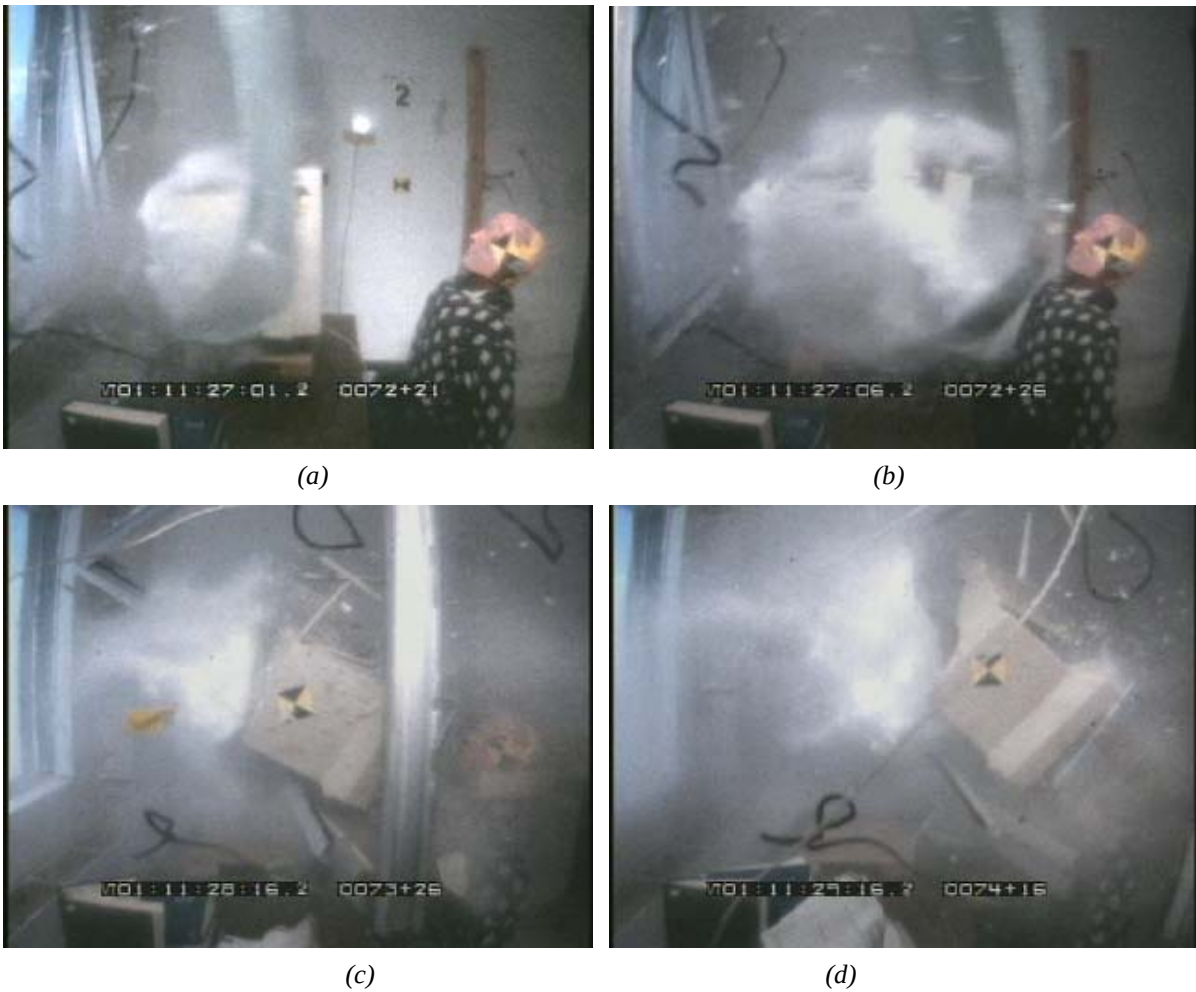
Figure 14. Snapshots from high-speed film of ATD behind computer monitor.
