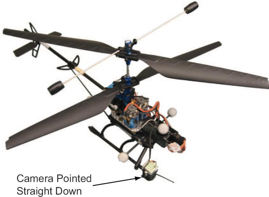
Figure 5: The Blade CX2 helicopter that was used for the experiments. It is a coaxial helicopter with a rotor diameter of 34.5 cms, a height of 18.3 cms and weighs approximately 220g (with battery).
