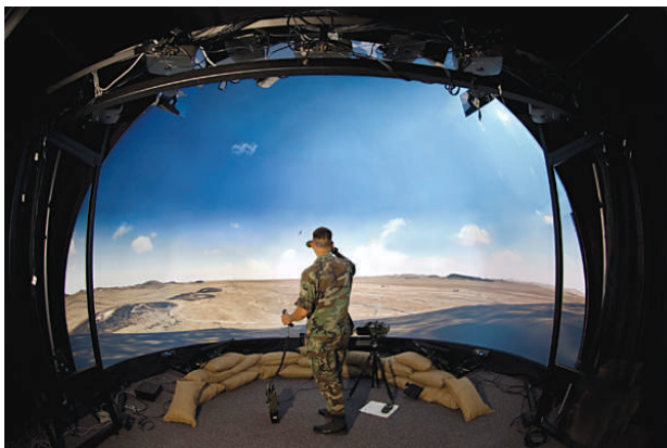
Figure 9. Visible wide-field-of-view projector system.
