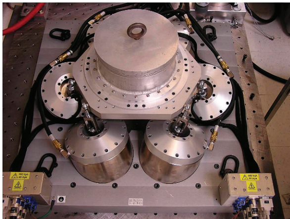
Figure 3. Five-axis high frequency Flight Motion Simulator table.
