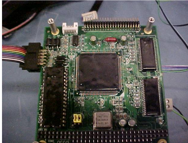
Figure 14. Video Graphic Adapter card. NOTE: Conformal Coated as described by Miller [19].
