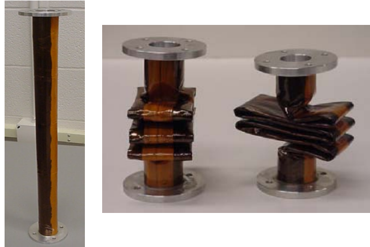
Figure 3. Rigidizable Inflatable Sub-Tg Tubes (20" long deployed) [14]
