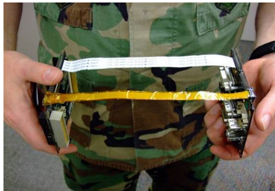
Figure 13. Kapton wrapped wire between user input board and processor board
