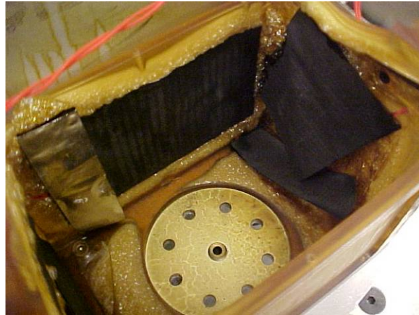
Figure 35. Damaged oven during Runaway Heater test
