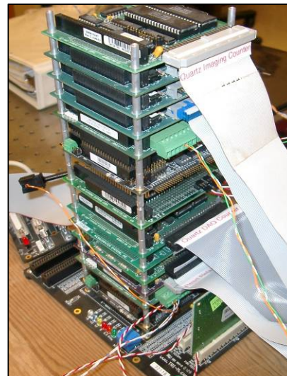
Moody's [6] two computer stack with 14 total PC-104 boards
