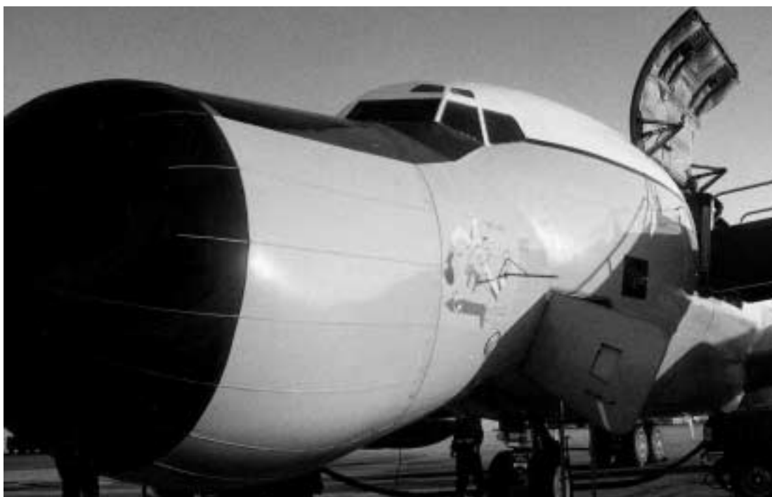
EC-135 Rivet Joint aircraft with "hog nose"
