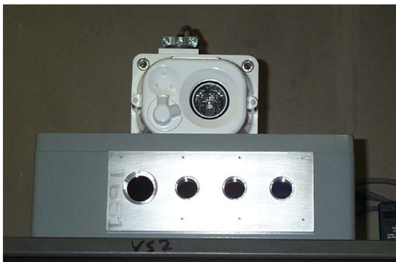
Figure 2-1 – Typical installation of the SBVS Component Prototype as tested in VS5 Test Series. The UV unit is positioned above the VIS/IR unit. See the text for a description of the individual elements.
