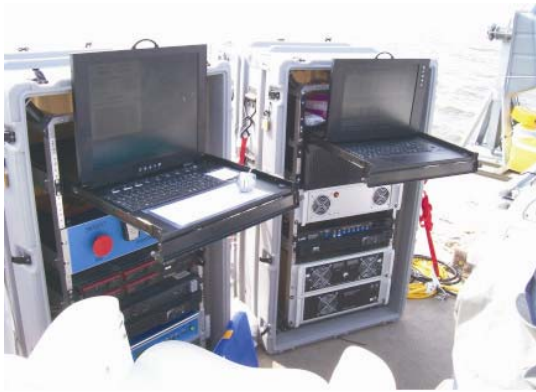
Figure 6. The two racks that control the sensor platform and all the data acquisition are shown. On the Coral Queen they will be located in the main cabin.
