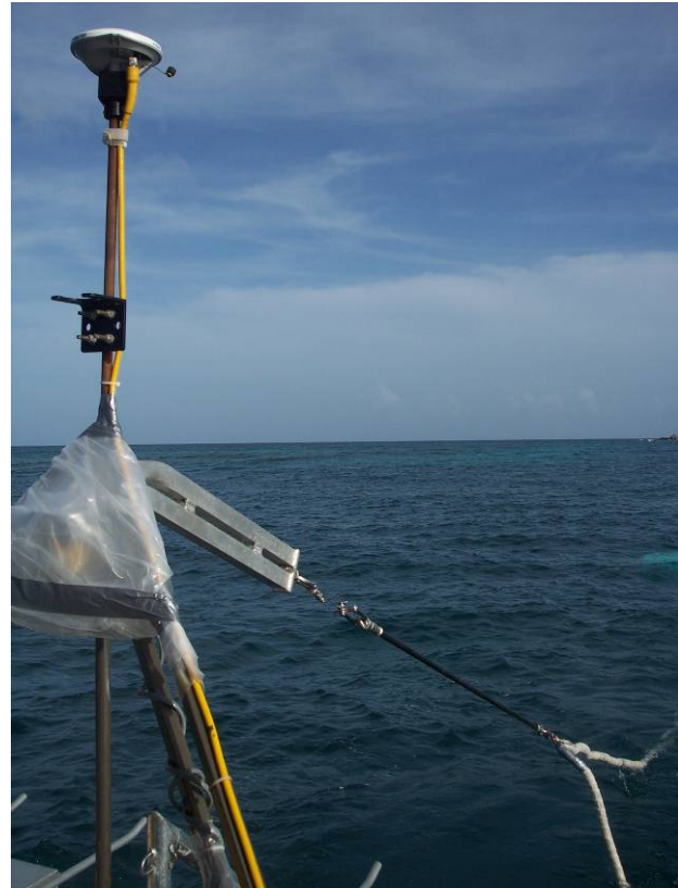
Figure 7-1. This image shows the weak link (mounted between the shackles at the end of the tow arm) and the Seaflex cable (the dark cable between the weak link and the tow cable).
