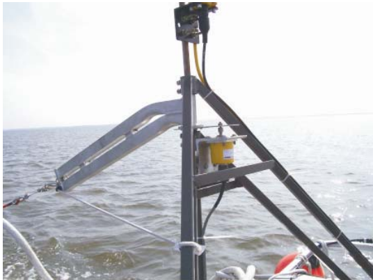
Figure 8. The tow arm assembly (with the weak link) is shown. Above the tow arm is the mount for the rear GPS unit.
