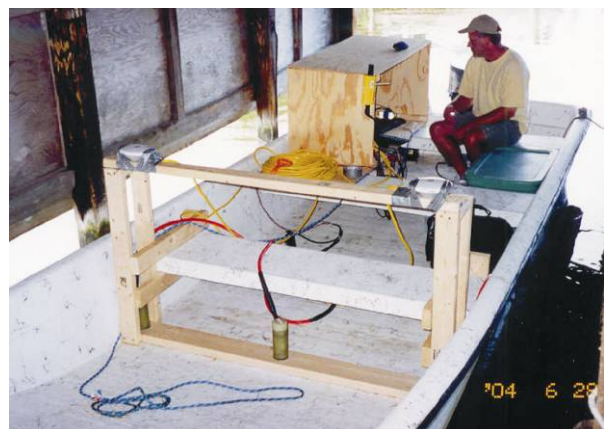
Figure 2-11. The 3-magnetometer array, GPS equipment, pilot guidance system, and data acquisition computers are shown mounted in the survey boat.
