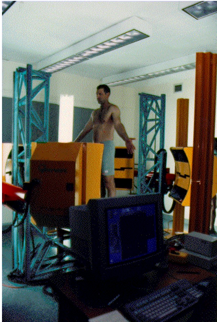
Figure 1-2. Subject being recorded on the Natick whole body laser scanner (courtesy of Brian Corner of Natick)
