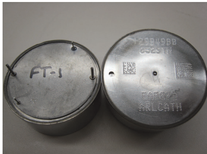
Figure 6. Enhanced liquid reserve MOFA battery prototypes.
