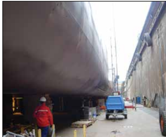
A Coast Guard Marine Inspector conducts a hull inspection on the new construction vessel OVERSEAS TEXAS at Aker Shipyard in Philadelphia, PA.
