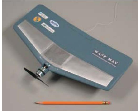
Figure 25. First generation DARPA Wasp micro air vehicle with polymer lithium-ion battery (silver quadrilaterals) integrated in composite wing skin structure [127].
