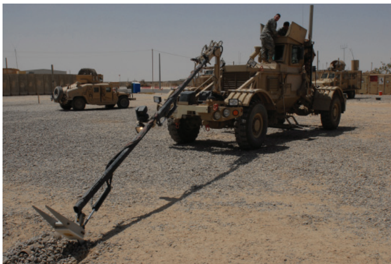
Photo 3: The Husky vehicle often served as the lead vehicle during route clearance mission. Equipped with an extended arm and camera, this one man vehicle often took the brunt of the EFP attacks during the battle of Sadr City. US Army photo by Spc. Opal Vaughn
