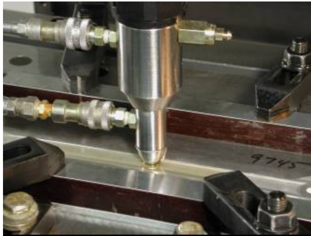
Figure 14 Low plasticity burnishing of a FSP 2219 aluminum plate.
