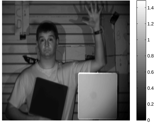
Figure 4.9: Estimated reflectance from Camera 2 using the raw data shown in Fig. 4.5 (Right).
