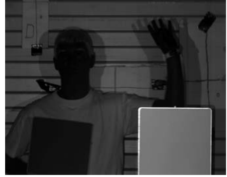
Figure 4.6: (Left) Raw image from the Goodrich SU640KTSX-1.7RT used for skin detection ( Camera 3 ) using the Semrock FF01-1060/13-25 filter. This configuration results in the light transmitting to ( Camera 3 ) as shown in Fig 3.33 (blue curve). (Right) Raw image from the Goodrich SU640KTSX-1.7RT used for skin detection ( Camera 4 ) using the Semrock NIR01-1570/3-25. This configuration results in the light transmitting to the ( Camera 4 ) as shown in Fig 3.34 (green curve).
