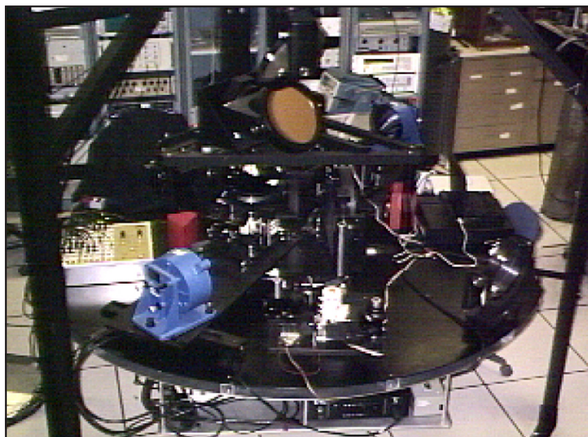
Open-loop rate table for hardware IRCM testing
