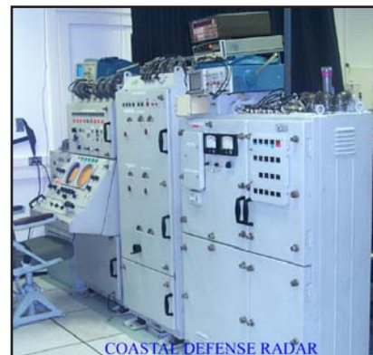
Search Radar ECM/EA Simulator (left), AN/SPS-66 PPI (center), and coastal defense radar (right)
