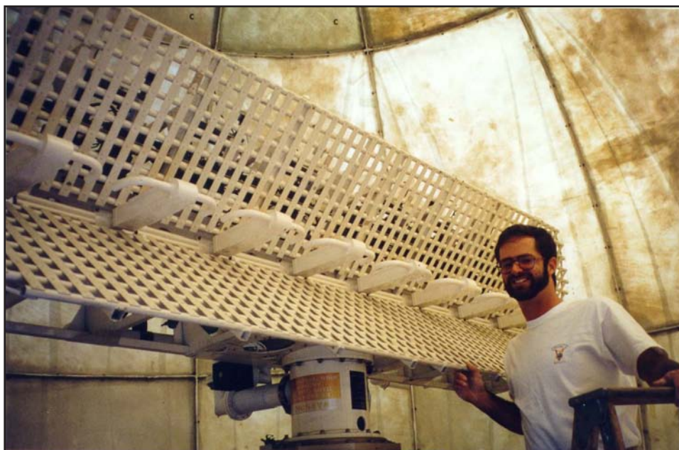
Ten-element AAFTE airborne radar array antenna
