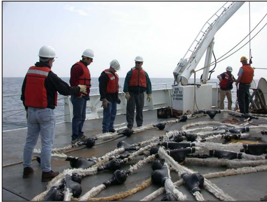
Preparing 64-element source/receive array for deployment
