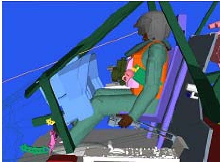
Figure 6 A clothed and equipped Jack mannequin in the Comanche helicopter (reproduced with permission)
