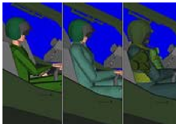
Figure 17: A mannequin in the Apache helicopter with a range of clothing and equipment (used with permission)
