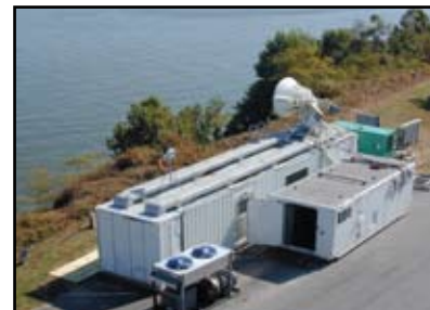
The W-band Advanced Radar for Low Observable Control (WARLOC) is a 94-GHz, high-power, coherent mmW radar.
