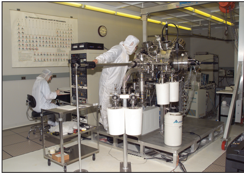
The Magnetoelectronics Fabrication Facility consists of a Class 1000 clean room equipped with tools for lithographic construction of magnetoelectronic and spintronic devices.
