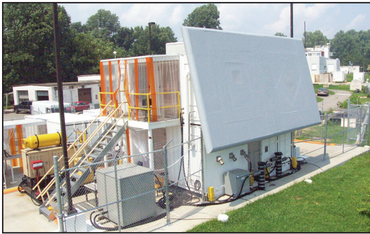
The AMRFC testbed, located at NRL's CBD, was developed as a proof-of-principle demonstration system that is capable of simultaneously transmitting and receiving multiple beams from common transmit and receive array antennas for radar, electronic warfare, and communications. These RF functions are controlled by common resource allocation manager (RAM) software over a real-time control network. New RF functionality may be readily added to the testbed as required for further demonstrations.
