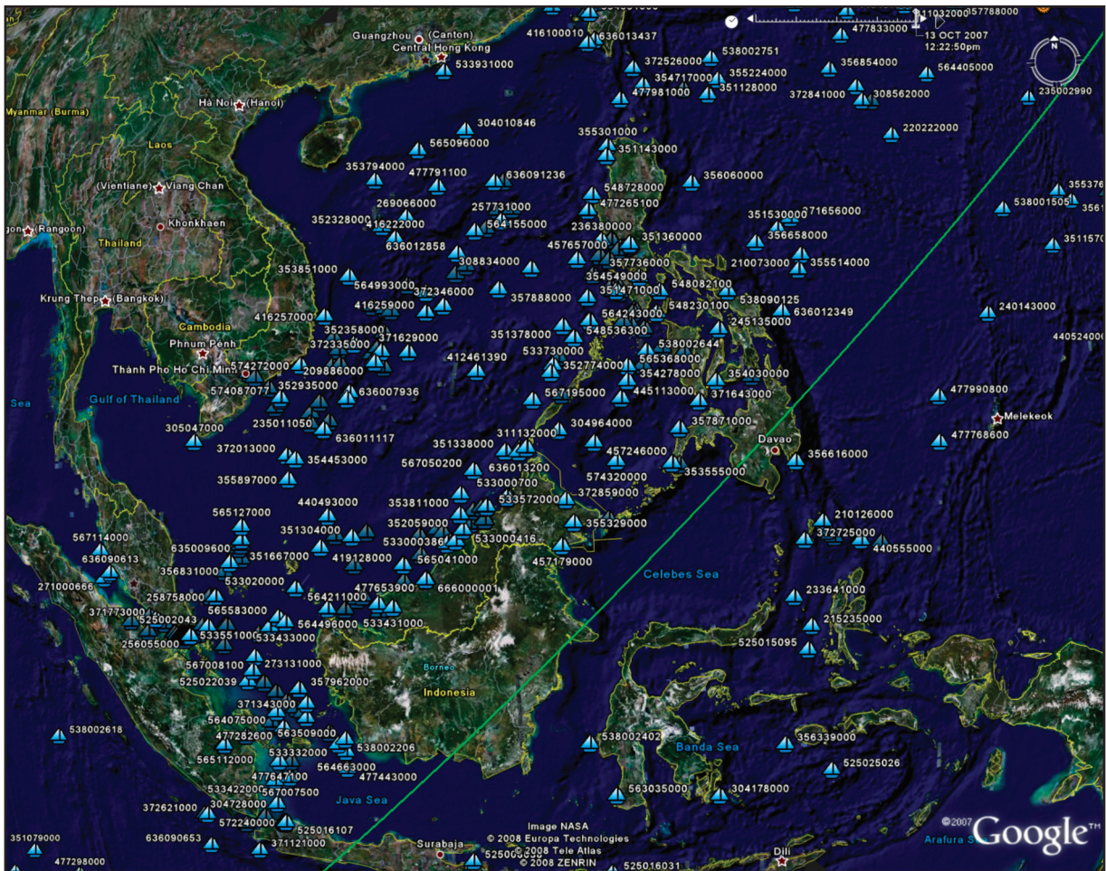
FIGURE 7 TIE AIS receiver performance in an area of high ship traffic density—South China Sea and Malacca Straits.
