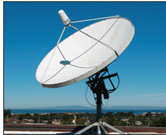
NRL's Marine Meteorology Division has a direct downlink capability for real-time geostationary data from NOAA's GOES-E and GOES-W satellites.
