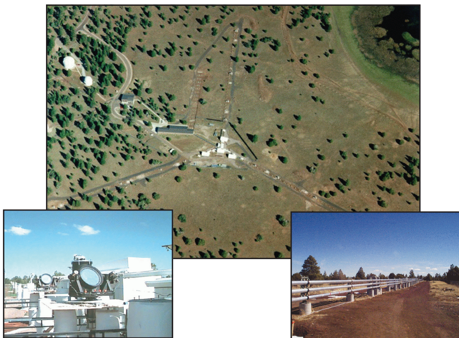
The Navy Prototype Optical Interferometer (NPOI) is used for operational astrometry and for development of distributed aperture imaging techniques.
