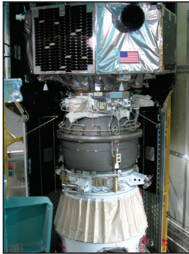
Left photo: Upper Stage spacecraft attached to Star48 3rd stage of Delta II 7925 booster. Right photo: MiTex/Upper Stage launch, 21 June 2006, 2215Z. (Courtesy USAF)
