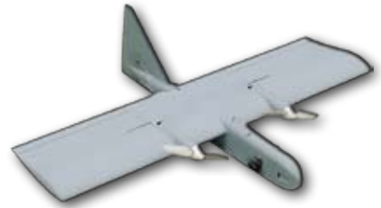
Dragon Eye unmanned air vehicle (UAV) system was designed, fabricated, tested with the warfighter, and transitioned to industry, and is another example of incorporating GPS into military platforms.
