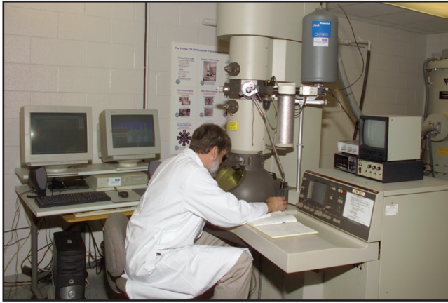
The Micro/Nanostructure Characterization Facility is capable of performing TEM, STEM, ARTEM, EELS, Z-contrast imaging, and spectral imaging.
