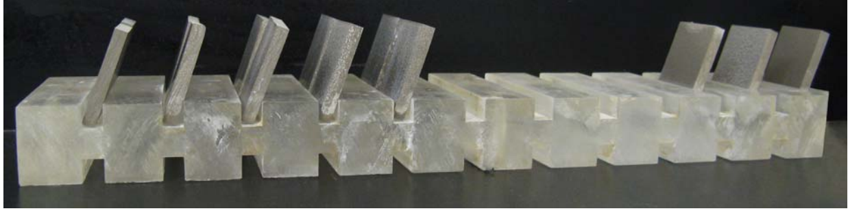
Figure 1. Corrosion rack configuration used for neutral salt fog (NSF) and GM 9540P exposures.
