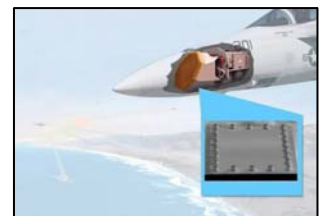
F/A-18 AESA Radar using die with Flip-Chip bumps
