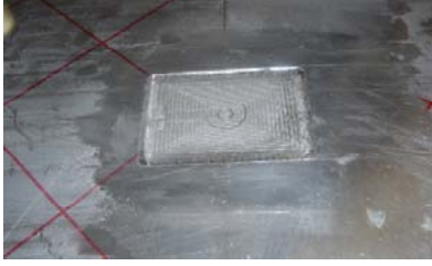
Figure 7 Simulated corrosion on aluminum plate.
