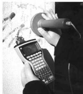
Corrosion activity being evaluated on a bridge wall with the GalvaPulse
