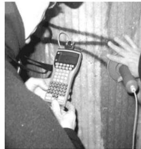
Highway bridge column being tested for corrosion rate with the GalvaPulse
