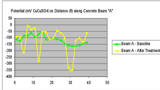
Figure 2d. Rebar half-cell potentials as a function of distance along beam "A" before and after treatment
