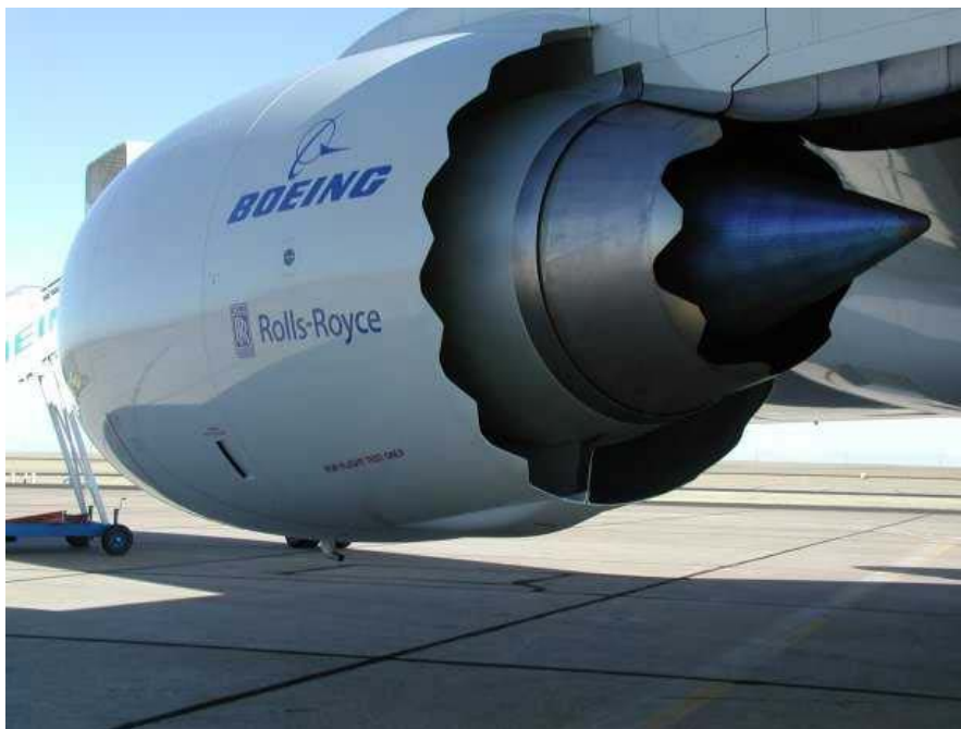
Figure 2.9: Flight Testing of Fixed Serrated Nozzle [2.127].
