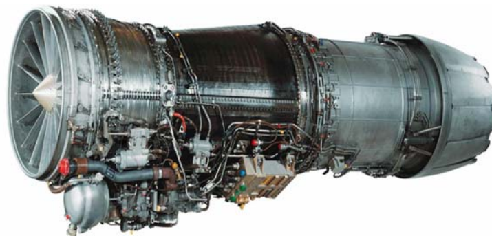
Figure 4.1: Engine Controls and Accessories Comprise a Substantial Portion of Total Engine Weight as Shown in this View of an F414 Engine.
