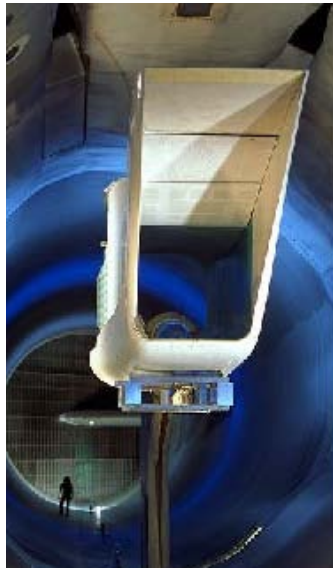
Figure 7.4: Boeing/SAMPSON Programme SMA Actuated Intake.
