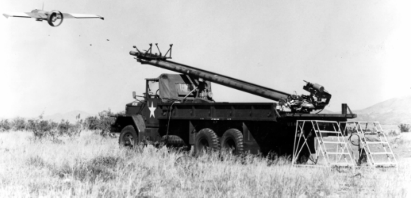
An Aquila remotely piloted vehicle is launched during testing at Fort Huachuca, Arizona, circa 1976.
