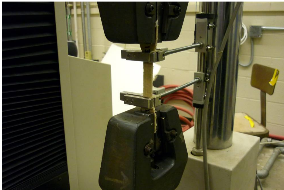
Figure 6.3 – Test Sample Mounted in Tensile Test Frame
