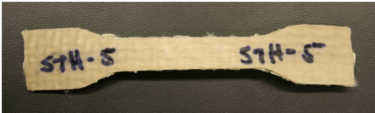
Figure 6.2 - Representative Tensile Coupon after Removal from Parent Hose Material
