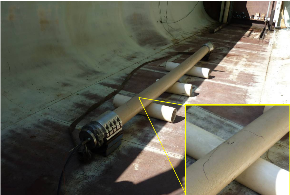
Figure 3.8 – Hose Sample E Burst Test Setup
