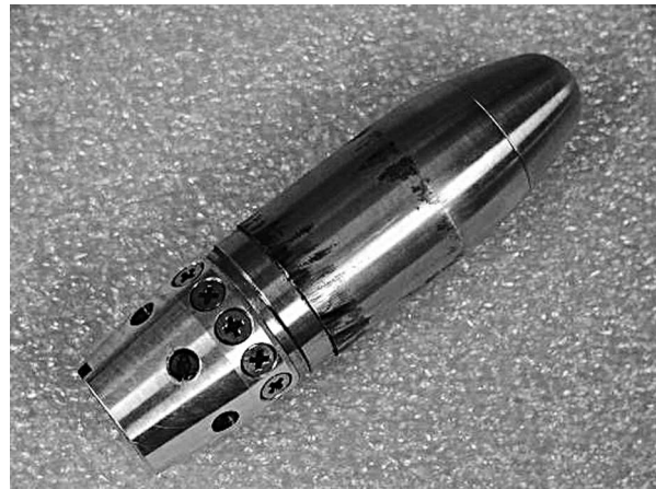
Figure 7. Recovered projectile after successful in-flight silicon chip bridge initiation
