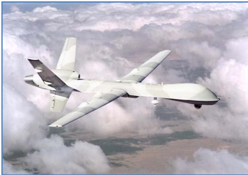
The Missile Defense Agency is examining the utility of airborne infrared sensors mounted on unmanned aerial vehicles to detect and track ballistic missiles.
