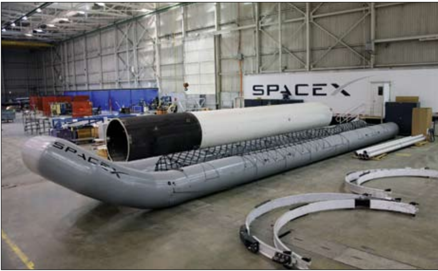
Figure 6. Falcon 1 recovery pontoon in front of the Falcon 1 first stage test unit. Upon locating the returned first stage, the recovery vessel will inflate and deploy the pontoon, strapping it around the stage and towing it back to port for refurbishment and reflight.
