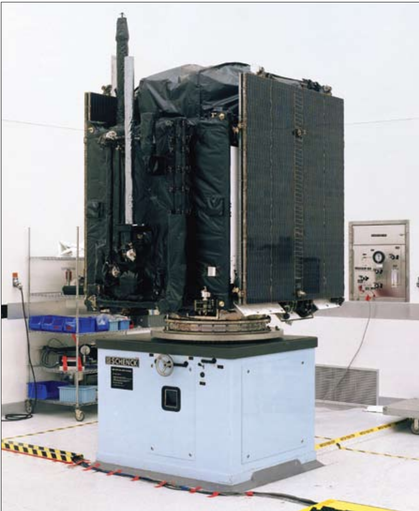
Figure 2. GPS IIR-18(M) Spacecraft on the Spin Table in the LCSS Spacecraft Processing Facility.
