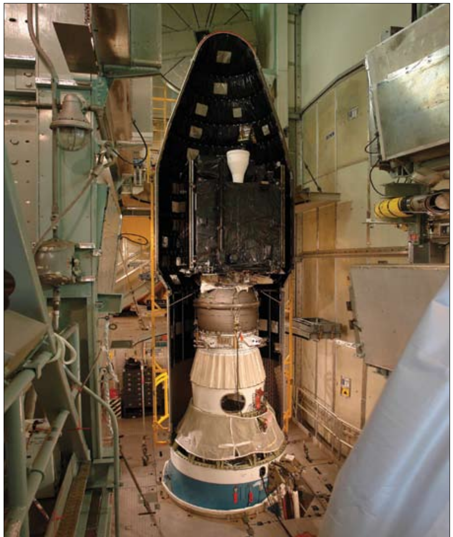
Figure 3. GPS IIR-18(M) Encapsulation at SLC-17.
