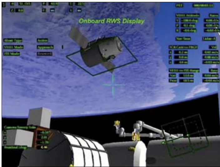
Figure 4. Computer simulation of Dragon spacecraft approaching the International Space Station.
