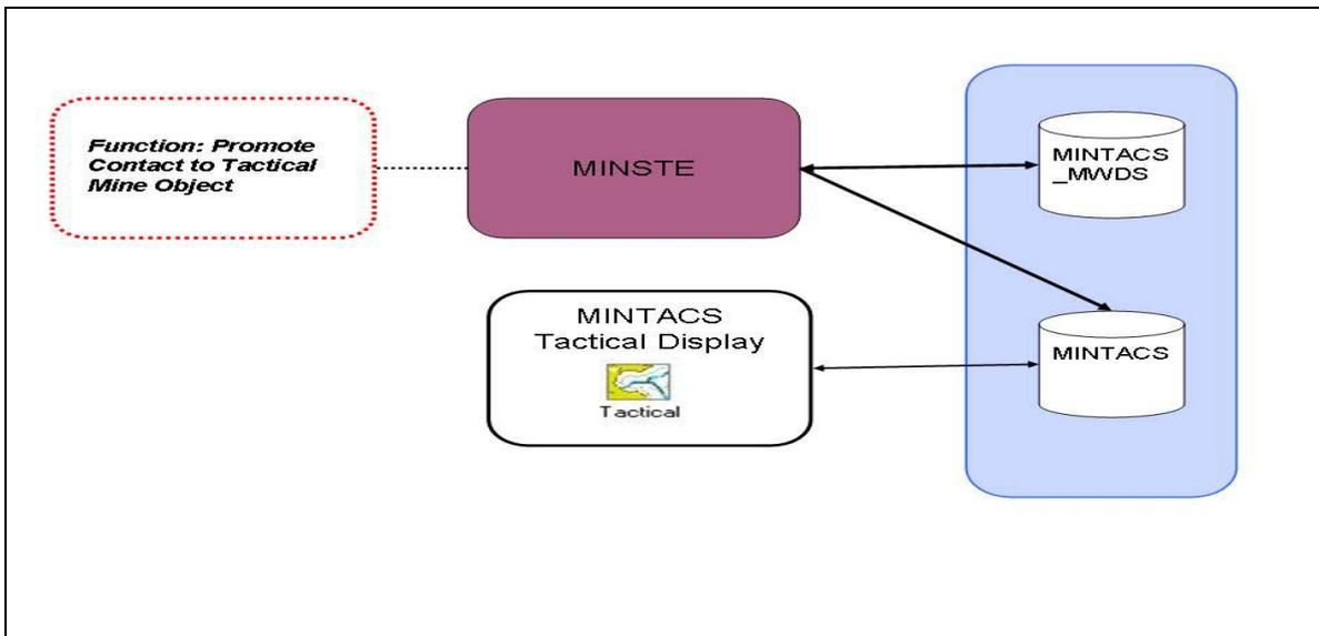
Figure 3: Diagram detailing MINSTE functionality. MINSTE communicates with the MINTACS RSDB, named MINTACS\_MWDS, to retrieve contact data to display to the user. The user is then able to select the contact to promote to be a Tactical Mine Object. MINSTE will format contact data into the correct data format to be imported into the MINTACS database, and be displayed as a mine object in the MINTACS Tactical Display.
