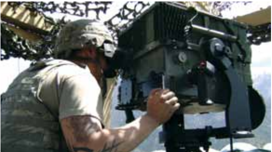
A Soldier from 173rd Airborne Brigade Combat Team using a Long-Range Advanced Scout Surveillance System in Operation Enduring Freedom to identify and locate enemy targets for an F-15.
