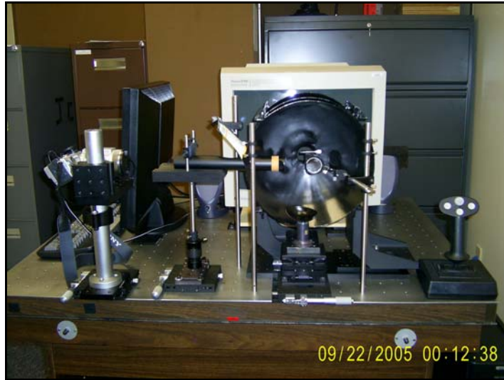
Figure 14. View of the glare tester from subject's perspective. Looking into the frustum nearest the subject the adjustable lens holder for the right eye can be seen along with the mirror-tube assembly allowing a continuous view of the left eye. The camera viewing the eye can be seen to the left. Corrective lenses, blur lenses, neutral density filters, fog and scatter plates, waveplates and artificial pupils were positioned in front of the right eye.
