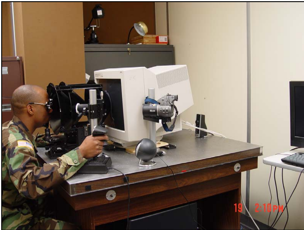
Figure 13. Subject position in glare tester. The subject views the monitor screen spot and glare annulus along the axis of three nested frustums. Subject responses are made using a joystick.
