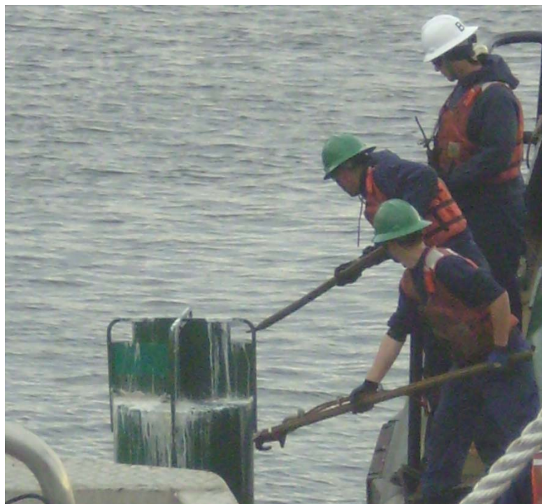
Figure B-7. Buoy recovery using boat hook and wire rope on pole.
