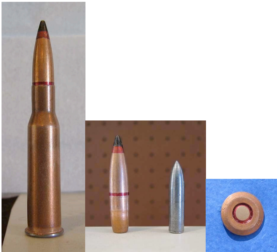
FIGURE 1. Cartridge, Bullet, Penetrator, and Headstamp of the 7.62-Millimeter x 54R Used in This Effort.
