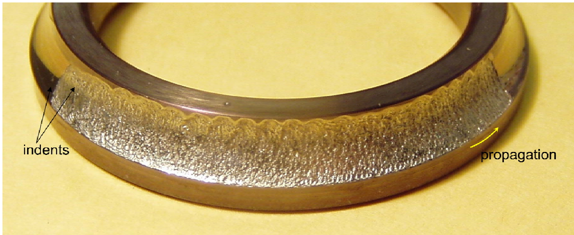
(a) Spalled M50NiL inner raceway
